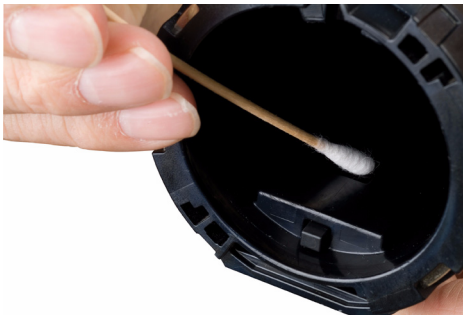
Fig. 21 Calibration cap diode cleaning
