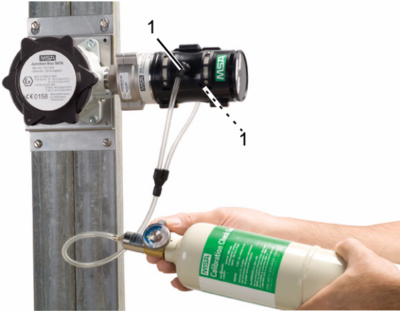
Fig. 15 HART calibration set-up
