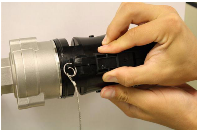
Fig. 18 Remove Environmental Guard
