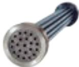
Straight cooler tubes, drawable to both sides of the cooler for easy cleaning and installation. The floating design prevent heat stress in the bundle and consequential damages.
